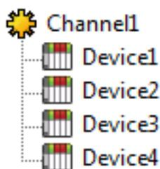
Each device appears under a single AutomationDirect EBC channel. In this configuration, the driver must move from one device to the next as quickly as possible in order to gather information at an effective rate. As more devices are added or more information is requested from a single device, the overall update rate begins to suffer.
