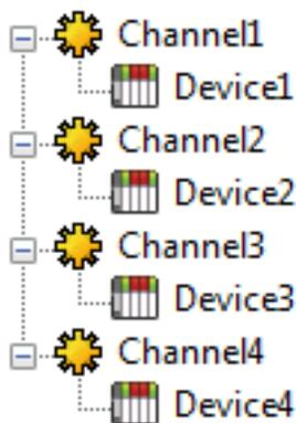
Each device has now been defined under its own channel. In this new configuration, a single path of execution is dedicated to the task of gathering data from each device. If the application has 100 or fewer devices, it can be optimized exactly how it is shown here.
