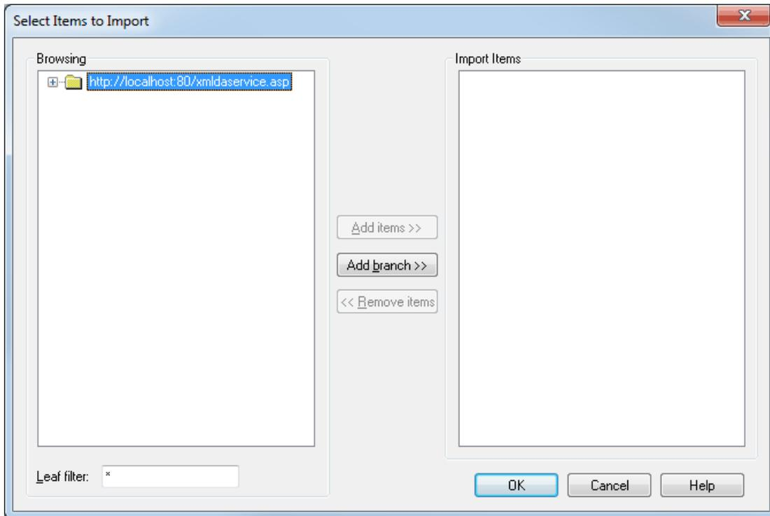
● **Note:** The Import Items list box only displays the list of tags that the user would like to import. The driver will validate the tags after the device has completed configuration. Any tags found invalid will not be created, and a message will be posted on the Event Log.
