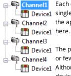
Each device has now been defined under its own channel. In this new configuration, a Device1 single path of execution is dedicated to the task of gathering data from each device. If the application has 256 or fewer devices, it can be optimized exactly how it is shown
