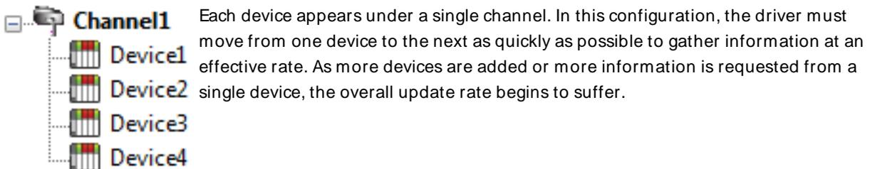
If the Yokogawa MX Driver could only define one single channel, then the example shown above would be the only option available; however, the Yokogawa MX Driver can define up to 100 channels. Using multiple channels distributes the data collection workload by simultaneously issuing multiple requests to the network. An example of how the same application may appear when configured using multiple channels to improve performance is shown below.
