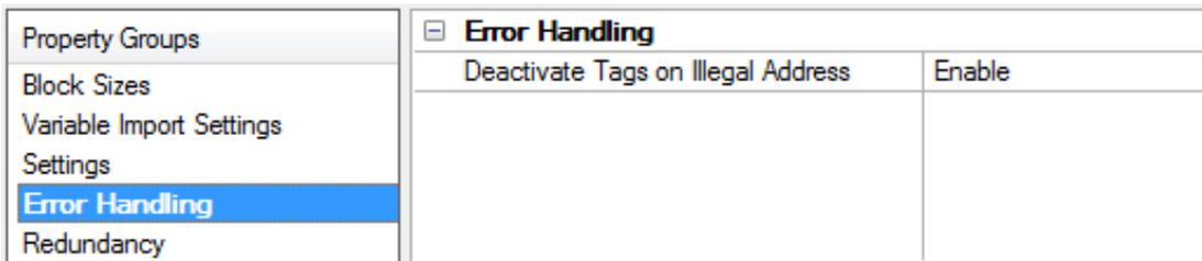
**Deactivate Tags on Illegal Address:** If a device returns Modbus exception code 2 (illegal address) or 3 (illegal data, such as number of points) in response to a read of a block, the driver can stop polling the block with the errors or continue trying to poll the block. Select Enable to stop polling on an illegal address error. Select disable to continue to poll that data block. Restarting the server is not required to activate a deactivated block. The default setting is enabled.
