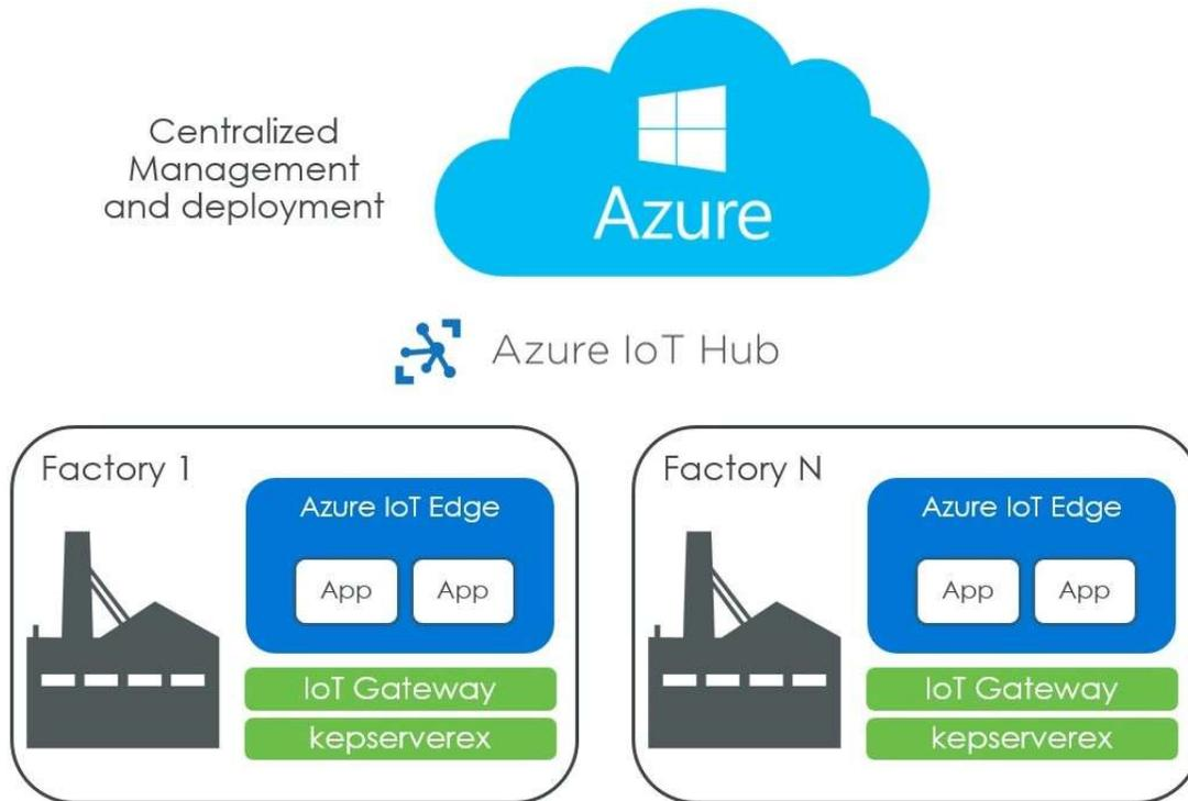
One textile manufacturer chose Microsoft and PTC to connect with multiple factories around the globe. One of their primary objectives was to track time on winding machines across multiple factories. KEPServerEX was already installed on these machines for connectivity, and they wanted to deploy Azure IoT Edge to their factory sites instead of sending data directly to the Azure IoT Hub.
