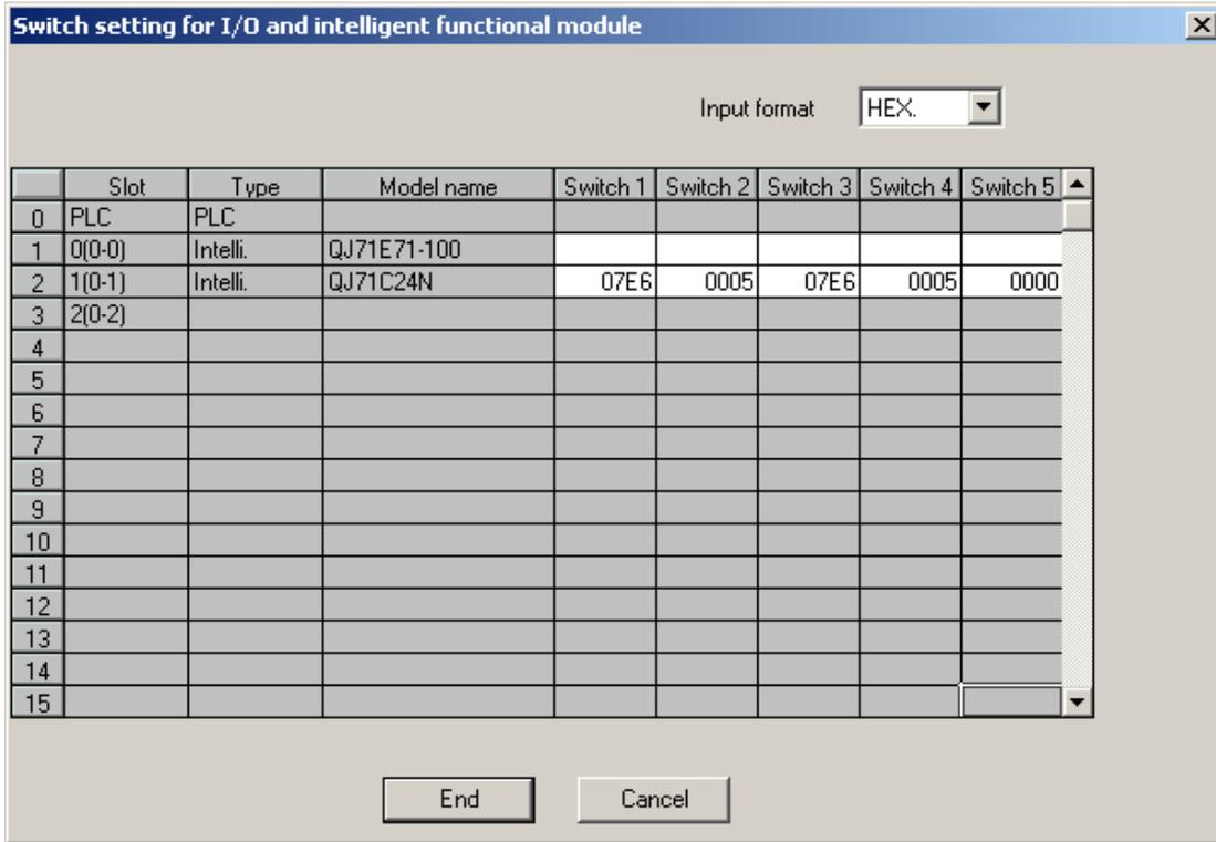
4. Entries for switch settings can be calculated from the following tables. Switches 1 and 2 are for channel 1 and switches 3 and 4 are for channel 2. For more information, refer to the tables and examples below.
