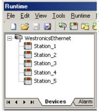
Each device appears under a single Thermo Westronics Ethernet channel. In this configuration, the driver must move from one device to the next as quickly as possible in order to gather information at an effective rate. As more devices are added or more information is requested from a single device, the overall update rate begins to suffer.
