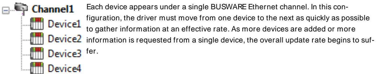
If the BUSWARE Ethernet Driver could only define one single channel, then the example shown above would be the only option available; however, the BUSWARE Ethernet Driver can define up to 100 channels. Using multiple channels distributes the data collection workload by simultaneously issuing multiple requests to the network. An example of how the same application may appear when configured using multiple channels to improve performance is shown below.
