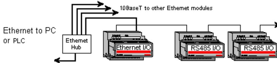
These intelligent Modbus interfaces accept Modbus Ethernet commands, convert them to traditional Modbus messages, and pass the command along to the RS485 port on the Ethernet interface. Replies from the station are returned to Modbus Ethernet format and passed back on the Ethernet network to the BUSWARE Ethernet I/O OPC Server.
