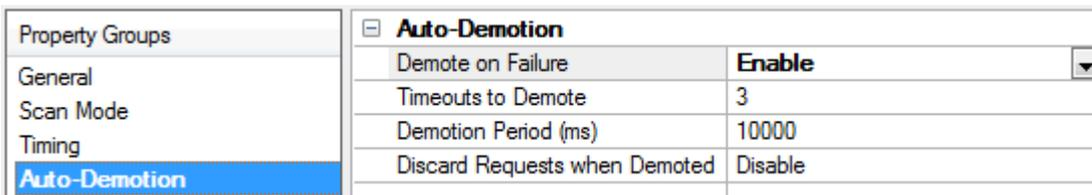
**Demote on Failure:** When enabled, the device is automatically taken off-scan until it is responding again.
