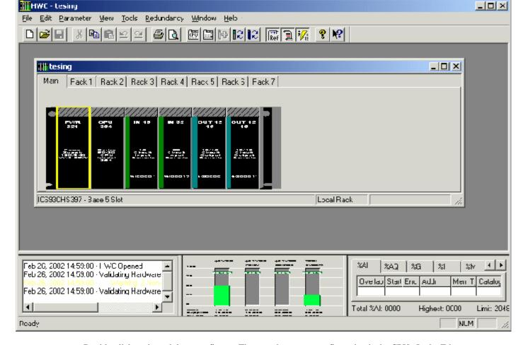
Double-click each module to configure. The most important configuration is the CPU. In the Ethernet tab of the CPU configuration window, the following parameters need to be configured:
