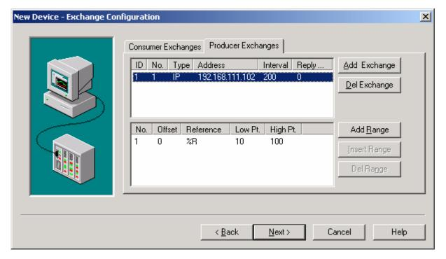
4. Next, click on the Producer Exchanges tab and add an exchange. Set the ID number to 1, the No. to 1, the Type to IP, and the address to the IP address of the PLC. **The value entered here for Producer Interval must match the value entered in VersaPro for Consumed Period.** Next, click "Add
