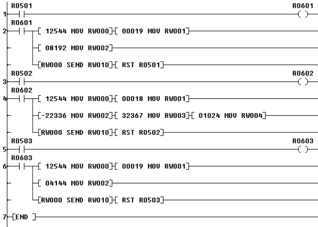
The first block of code at rung 2 places the PLC in Standby Mode when bit R0501 is set. This must be done before the IP and port can be set. The second block of code at rung 4 sets the IP and port number when bit R0502 is set. The final block of code at rung 6 puts the PLC back in Run Mode when bit R0603 is set.
