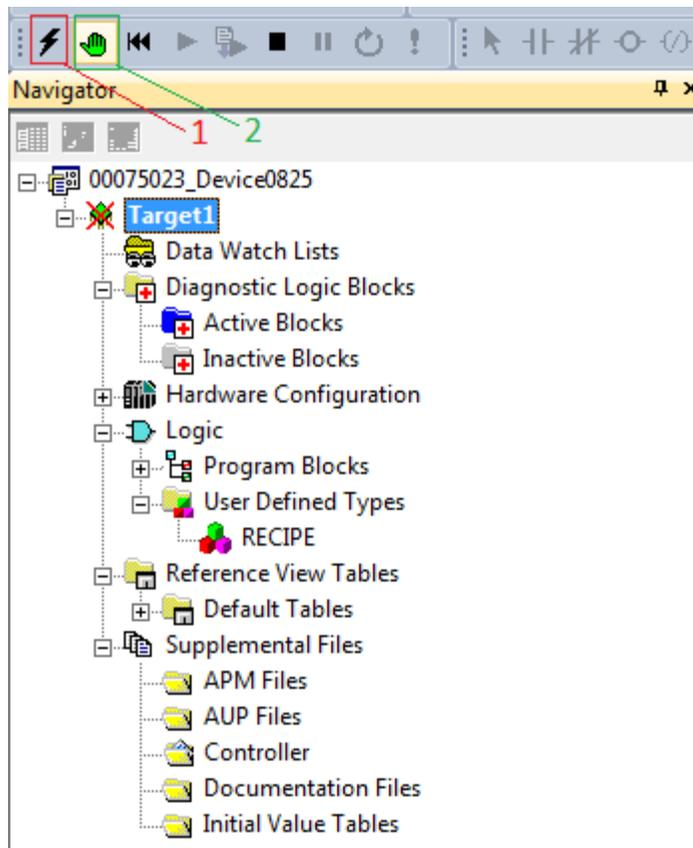
7. When the target should turn green with a red X on the target as the project in the controller does not match the project in Proficy ME.
