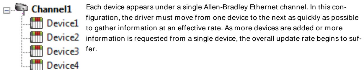
If the Allen-Bradley Ethernet Driver could only define one single channel, the example above would be the only option available; however, the driver can define up to 256 channels. Using multiple channels distributes the data collection workload by simultaneously issuing multiple requests to the network. An example of how the same application may appear when configured using multiple channels to improve performance is shown below.
