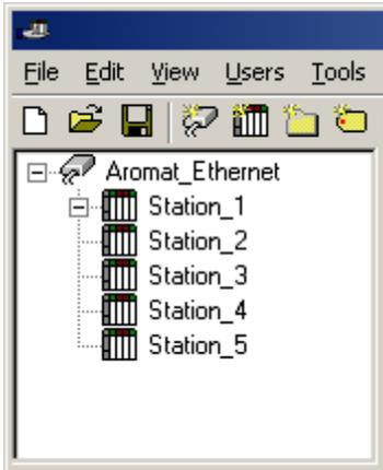
Each device appears under a single Aromat Ethernet channel. In this configuration, the driver must move from one device to the next as quickly as possible in order to gather information at an effective rate. As more devices are added or more information is requested from a single device, the overall update rate begins to suffer.
