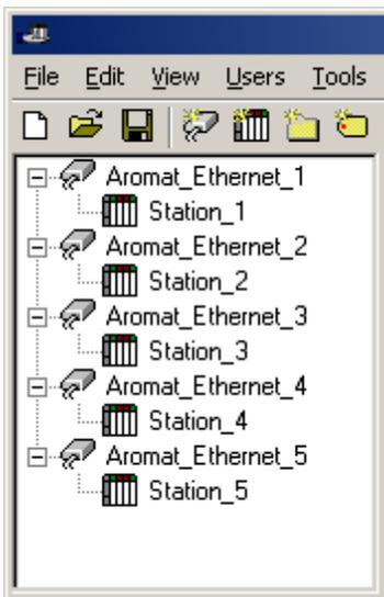
Each device has now been defined under its own channel. In this new configuration, a single path of execution is dedicated to the task of gathering data from each device. If the application has 16 or fewer devices, it can be optimized exactly how it is shown here.
