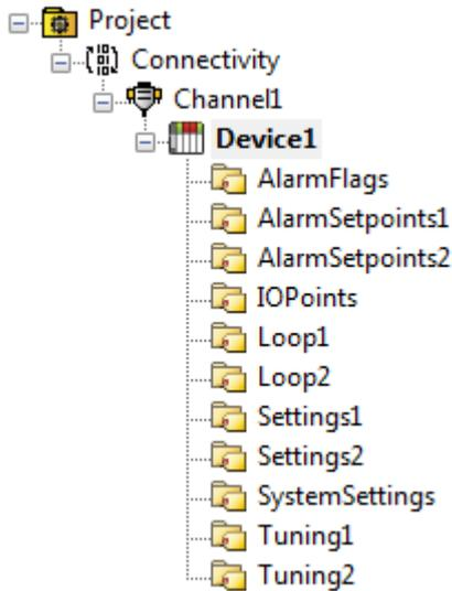
The Yokogawa YS100 Driver utilizes the OPC server's Automatic Tag Database Generation feature by automatically creating tags through the use of a fixed database. When a device model is selected, tag and tag group generation will occur. The image below displays the results of Automatic Tag Database creation for a YS150 device.
