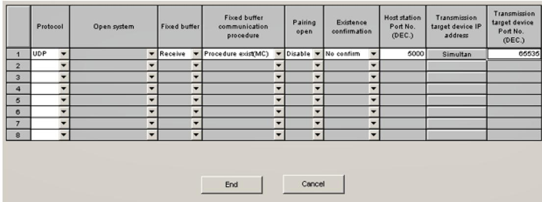
**Write Network Parameters to PLC**
