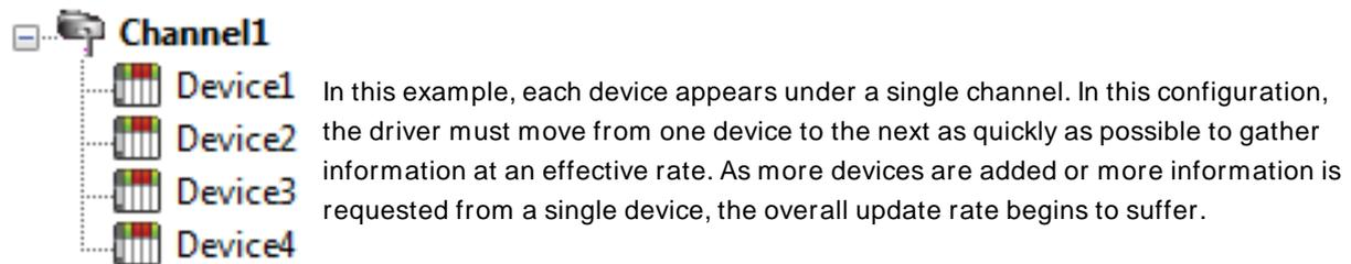
If the CODESYS Driver could only define a single channel, the example above would be the only option. However, the driver can define up to 1024 channels. Using multiple channels distributes the data collection workload by simultaneously issuing multiple requests to the network. An example of how the same application may appear when configured using multiple channels to improve performance is shown below.
