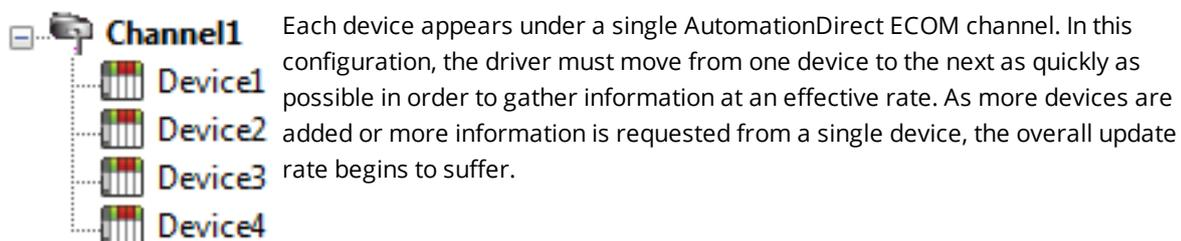
If the AutomationDirect ECOM Driver could only define one single channel, then the example shown above would be the only option available; however, the AutomationDirect ECOM Driver can define up to 16 channels. Using multiple channels distributes the data collection workload by simultaneously issuing multiple requests to the network. An example of how the same application may appear when configured using multiple channels to improve performance is shown below.
