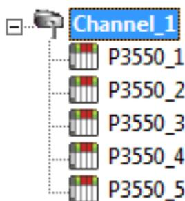
Each device appears under a single channel. In this configuration, the driver must move from one device to the next as quickly as possible to gather information at an effective rate. As more devices are added or more information is requested from a single device, the overall update rate begins to suffer.
