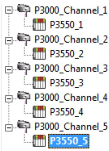
Each device can be defined under its own channel. In this configuration, a single path of execution is dedicated to the task of gathering data from each device. If the application has 100 or fewer devices, it can be optimized exactly how it is shown here.
