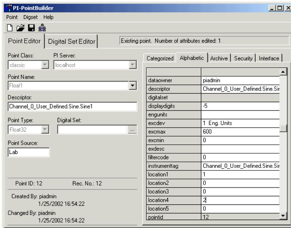
7. Next, copy the **instrumenttag** data and add it to **Descriptor**. This provides a description of the tag.
