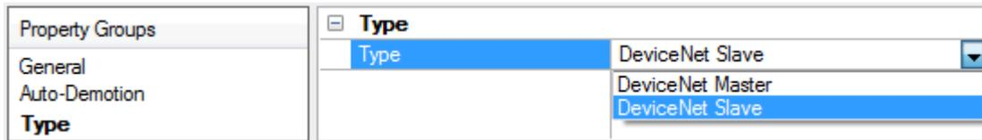
**Type:** When applicable, this property defines the device's bus type and master/slave type. Supported device types include DeviceNet Master, DeviceNet Slave, Profibus-DP Master, and Profibus-DP Slave.
