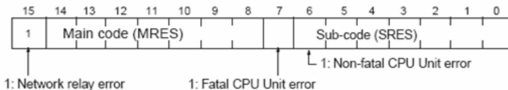
If bit 6 or 7 is ON, an error has occurred in the destination CPU unit. If this occurs, refer to the operation manuals for the CPU unit where the error occurred and then remove the cause of the error.
