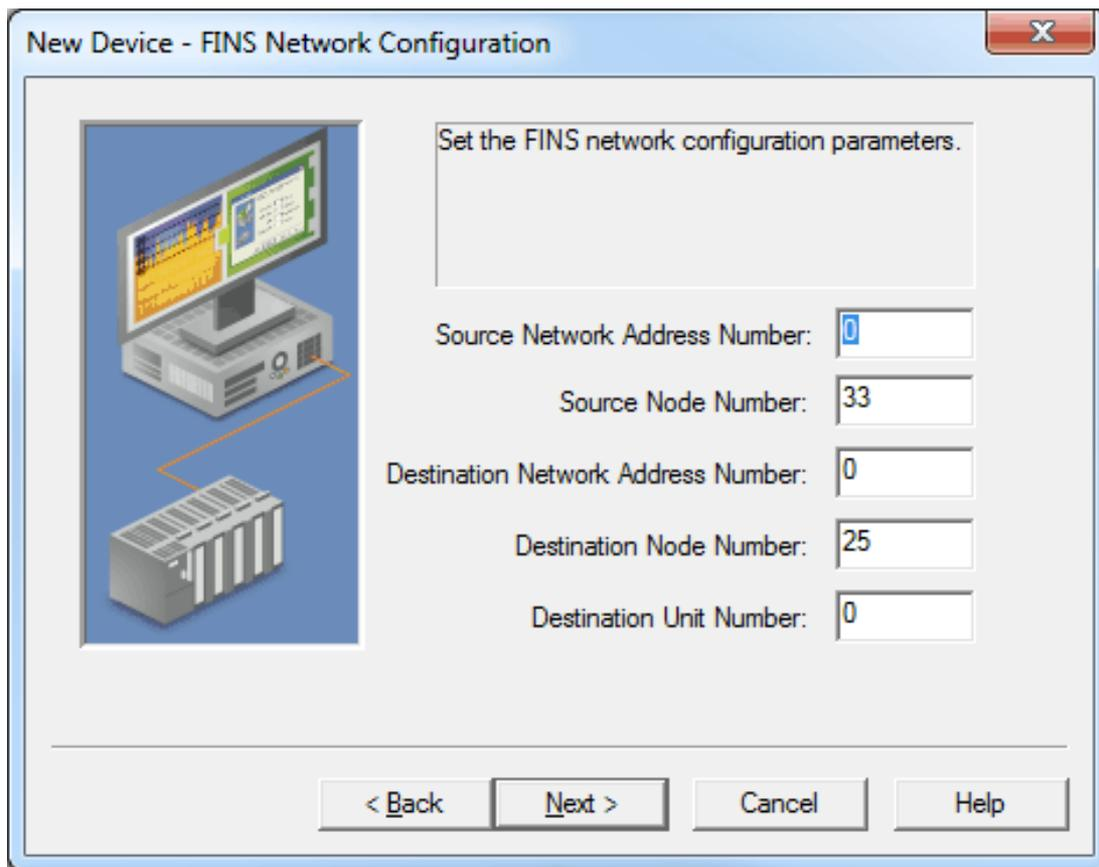
The default value for network addresses is zero. This is interpreted by FINS as instruction to use the local network. Actual network numbers can range from 1 to 127. Using zero is convenient if there is only one network level. When using gateway devices, however, specify the actual network number (1–127) to avoid routing ambiguities.
