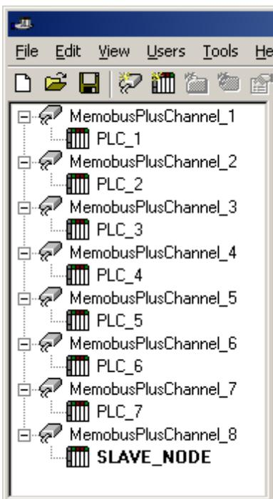
Each device has now been defined under its own channel. In this new configuration, a single path of execution is dedicated to the task of gathering data from each device. If the application has 8 or fewer devices, it can be optimized exactly how it is shown here.
