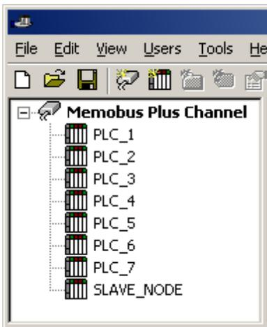
Each device appears under a single Yaskawa MemobusPlus channel. In this configuration, the driver must move from one device to the next as quickly as possible in order to gather information at an effective rate. As more devices are added or more information is requested from a single device, the overall update rate begins to suffer.
