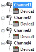
Each device has now been defined under its own channel. In this new configuration, a single path of execution is dedicated to the task of gathering data from each device. If the application has 32 or fewer devices, it can be optimized exactly how it is shown here.
