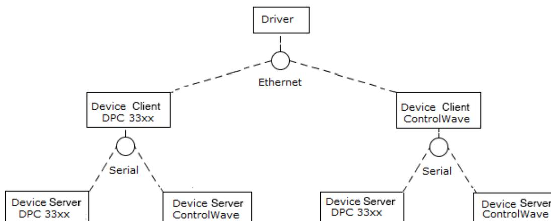
The Bristol/IP Driver communicates to Client or Server devices using Ethernet (UDP). Communications to Client devices are direct: the driver sends a request to the device and it responds. Communications to server devices are indirect: the driver sends a request through the client device. In most configurations, server devices communicate over serial to the client.
