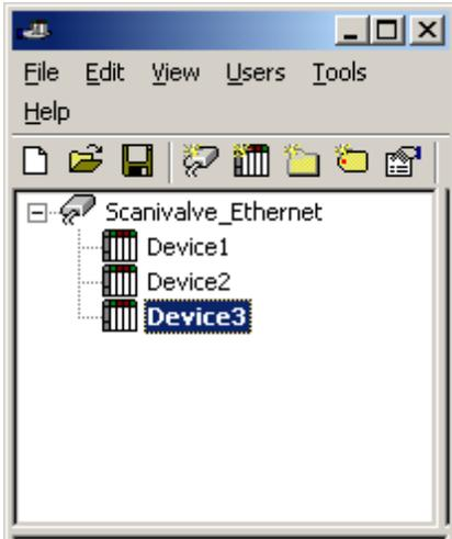
Each device appears under a single Scanivalve Ethernet channel. In this configuration, the driver must move from one device to the next as quickly as possible in order to gather information at an effective rate. As more devices are added or more information is requested from a single device, the overall update rate begins to suffer.
