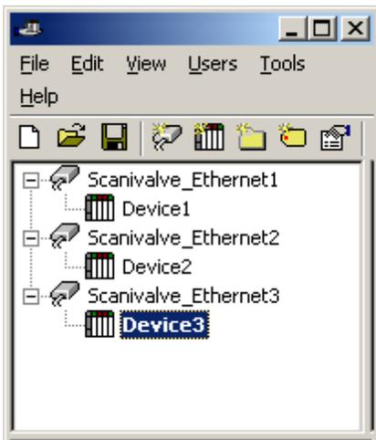
Each device has now been defined under its own channel. In this new configuration, a single path of execution is dedicated to the task of gathering data from each device. If the application has 100 or fewer channels, it can be optimized exactly how it is shown here.
