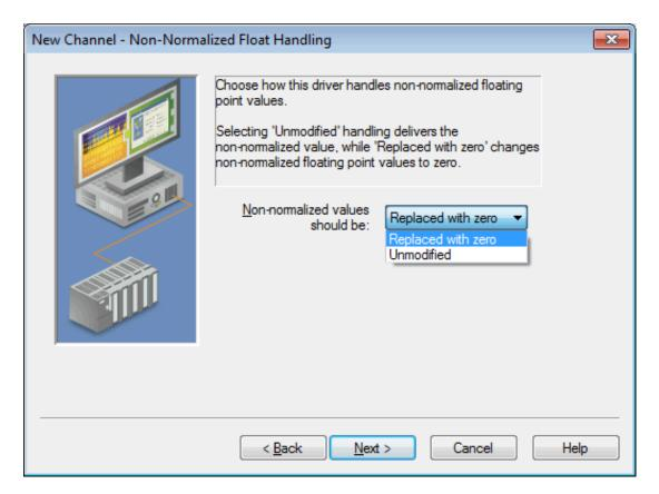
**Replaced with zero** recognizes invalid outliers and eliminates them by replacing the value with integer zero (default).
