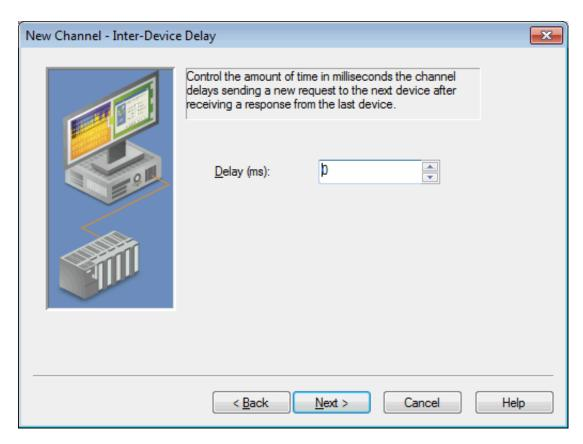
**Delay** Accept 0 milliseconds (default) or adjust using the up/down arrows. The range is 0-60000 ms.
