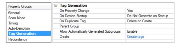
On Property Change: If the device supports automatic tag generation when certain properties change, the On Property Change option is shown. It is set to Yes by default, but it can be set to No to control over when
