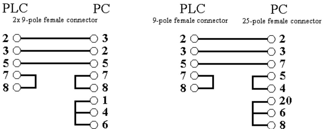
**Cable Connections for a PC20 Model Device**
