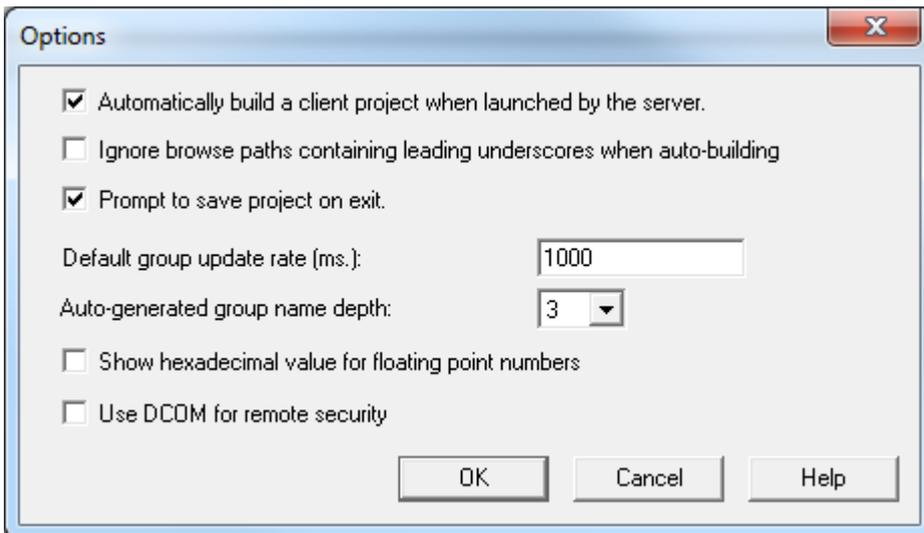
**Automatically Build a Client Project When Launched by the Server:** When checked, the OPC Quick Client will automatically build a client project with all the tags in the OPC server when it is launched from the OPC server. The default setting is checked.
