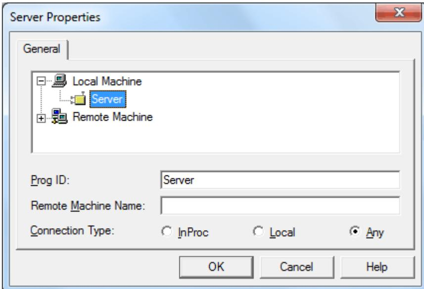
**Prog ID:** This parameter specifies the Prog ID of the OPC Server to which the client will connect. Use the tree display to browse for registered servers. The Prog ID field can be automatically updated by double-clicking on any registered server.
