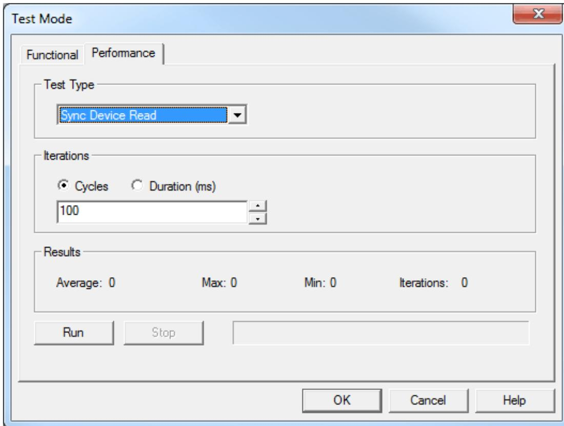
**Test Type:** This parameter specifies the test type. Tests are named after the operation that they perform. Options include Sync Device Read, Sync Cache Read, and Sync Write (which writes a random value to each item). The default setting is Sync Device Read.
