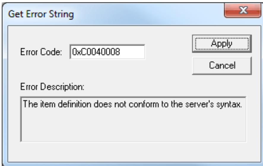
● **Note:** To request an error description from the server, enter the error code and then press **Apply**. If the server can translate the error code, the description will appear. An OPC server should be able to translate any OPC error code, in addition to Win32 errors.
