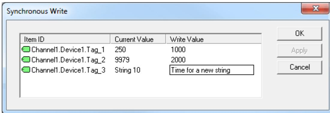
● **Note:** Both types of writes utilize the same dialog. The dialog displays the current value at a 100 millisecond refresh rate. To send the data to the server, enter the data to write in the Write Value column and then press **Apply**. To apply the write and close the dialog, click **OK**. To abort the operation, click **Cancel**.
