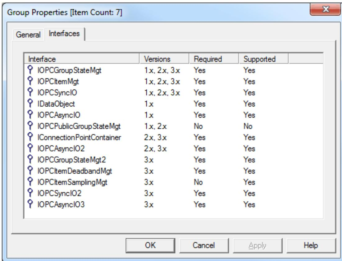
**Note:** Interfaces that are not required are considered optional. The Supported column states which group interfaces are supported by the server.
