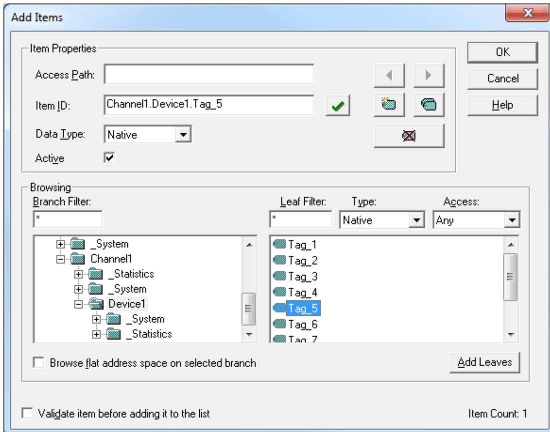
**Access Path:** This parameter is required by some OPC servers to complete an item definition. To determine whether an access path is needed, refer to the OPC server's help documentation.
